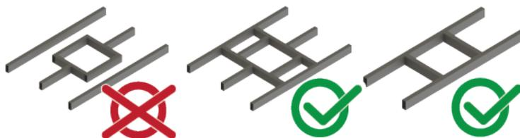
3. The opening created must be framed to provide adequate support and prevent air from being drawn from the roof cavity.
